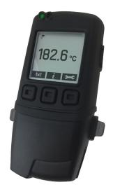
This standalone data logger measures and stores more than 250,000 temperature readings from a K, J or T-type thermocouple at a resolution of  $0.1^{\circ}$ C ( $0.2^{\circ}$ F). It comes supplied with a K-type thermocouple capable of measuring from -80 to +400°C (-112 to +752°F).
