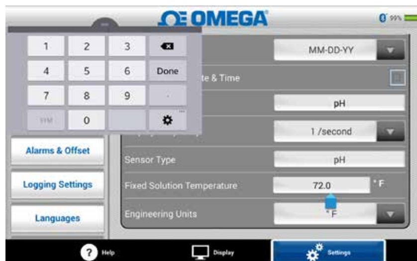
Figure 5-37. Setting Fixed Temperature For Solution
