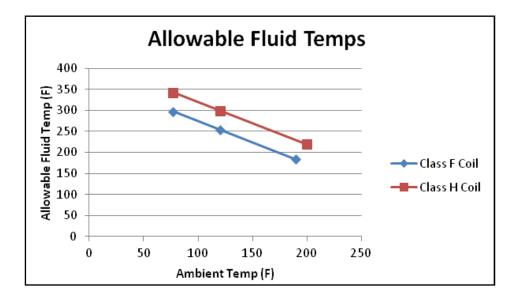
If the coil is only being powered intermittently for short periods of time, the allowable fluid temperature is 400°F when in an ambient temperature of 77°F.
