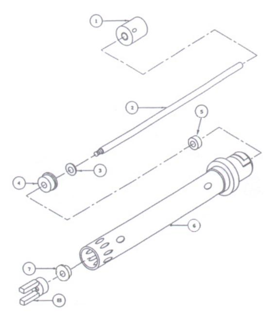
**Generator Probe Replacement Parts**
