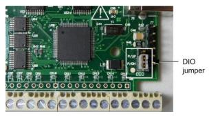
Figure 5. Pull-up/down jumper location
