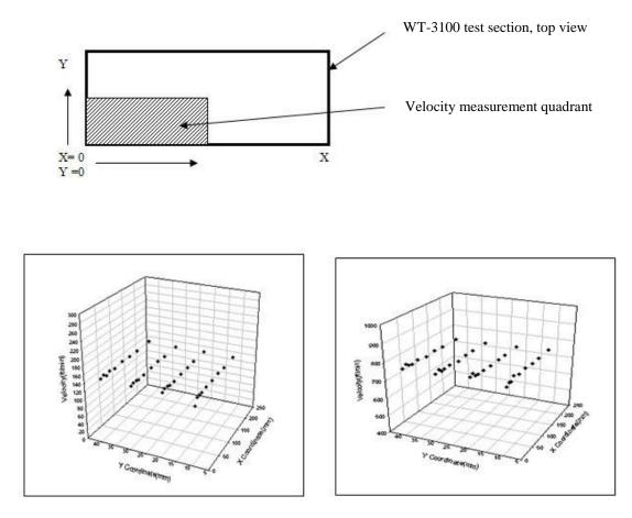
Velocity Distribution for one quadrant of the WT-3100 Wind Tunnel Cross Section at 150 ft/min
