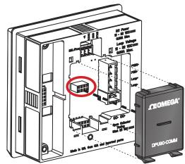
Enables communication with a HART<sup>®</sup>-enabled device. See DPU91 product manual pg. 10-17 for additional information.
