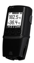
The OM-EL-GFX-DTC standalone USB data logger measures and stores up to 252,928 temperature readings from two J, K, or T-type thermocouple inputs at a resolution of 0.1°C/0.1°F. Using the Windows control software (available as a free-download from www.omega. com), users can quickly set up the data logger and view downloaded data by connecting the device to the PC's USB port using the supplied cable.
