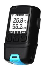
The OM-EL-GFX-2 standalone USB data logger measures and stores up to 252,928 temperature and humidity readings over a -30 to  $+80^{\circ}$ C (-22 to  $176^{\circ}$ F) and 0 to 100% RH range at a resolution of  $0.1^{\circ}$ C/ $0.1^{\circ}$ F and 0.1% RH. Using the Windows control software (available as a free download from www.omega.com), users can quickly set up the data logger and view downloaded data by connecting the device to the PC's USB port using the supplied cable.
