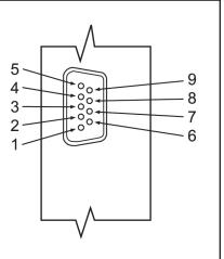
FIGURE 2.a - 9-PIN "D" CONNECTOR PINOUTS FOR FMA1700A/1800A TRANSDUCER
