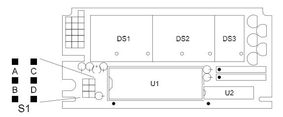
Figure 5.1 Display Board Jumper Locations
