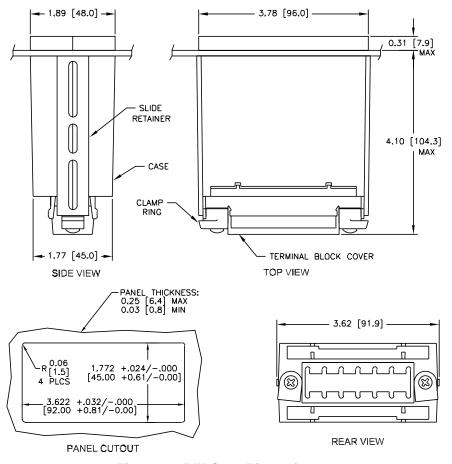
Figure 3.1 DIN Case Dimensions
