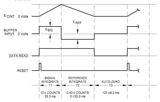
Figure 8.1 Dual-slope Conversion Diagram
