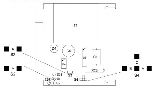
**Figure 5.2 Main Board Jumper Locations**
