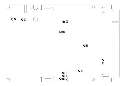
Figure 5.3 Solder Switch Locations
