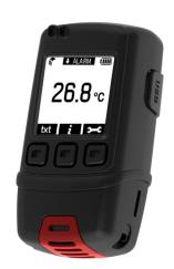
The OM-EL-GFX-1 standalone USB data logger measures and stores up to 251,928 temperature readings over a -30 to +80°C (22 to +176°F) range and at a resolution of 0.1°C (0.1°F). Using the Windows control software (available as a free-download from www.omega.com), users can quickly set up the data logger and view downloaded data by connecting the device to the PC's USB port using the supplied cable.
