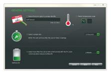
3 Name your Sensor, Select Temperature Scale, Sample Rate & Transmission Rate
