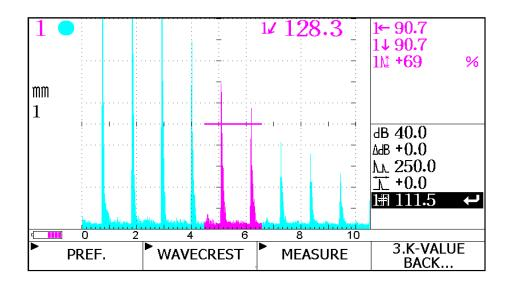
Figure 14. Calibration Interface of the Probe's K Value
