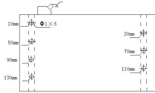
Figure 23a. CSK-III Test Block
