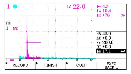
Figure 24. Creating and Recording the First Point of the DAC Curve
