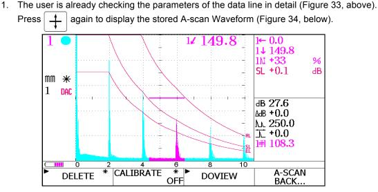
Figure 34. Screen Shot: A-Scan Waveform
