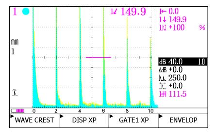
Figure 21. Envelop Function – Main Screen
