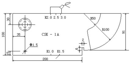
CSK-I Test Block of Measuring the Probe's K Value
