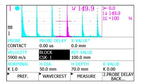
Figure 13. Adjusting Parameters for Calibrating Delayed Time
