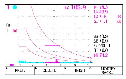
Figure 26. Modifying the DAC Curve
