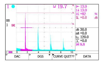
Figure 30. The DAC or AVG Curve Menu Screen - "Curve Quit ??" Exit Shortcut Location
