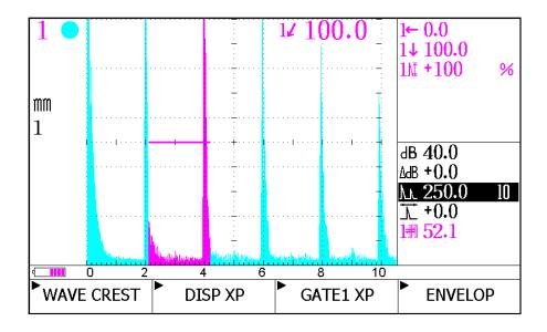
Figure 4. Display Interface of the BASIC Flaw Detection
