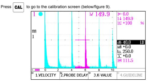
Figure 9. Calibration Display Screen
