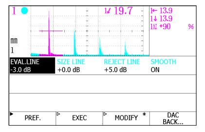
Figure 23. Main Menu – Adjustable Parameters, DAC Curve
