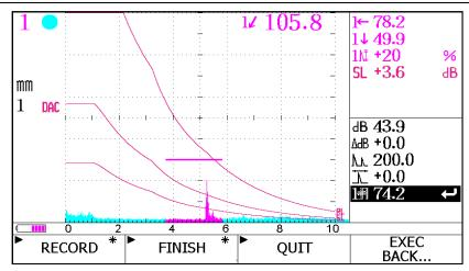
Figure 25. The DAC Curve Finished Results
