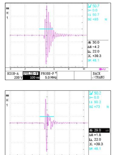
A.3 The sensitivity is the best when the width of the square-wave is a cycle of probe frequency (for example, 5MHz corresponds to approximately 210ns).
