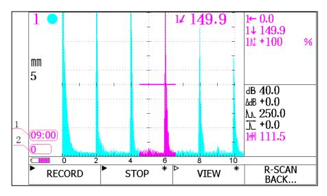
Figure 37. "Recording Waveform Data" Screen Shot1. Available Recording time2. Number of Recorded Frames
