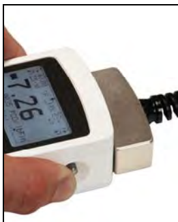
Fig. 3.2 Press both buttons on either side of the indicator housing to release the connector.
