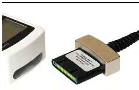
Fig. 3.1 Appropriate orientation of the connector.
