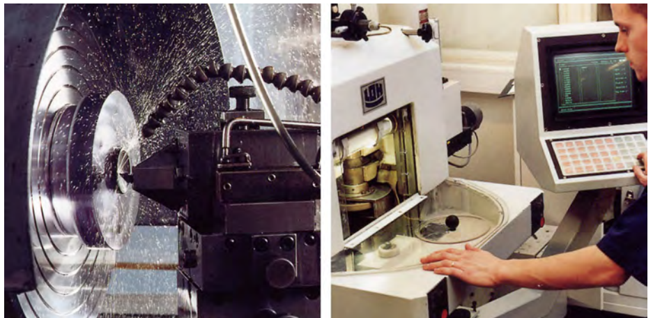
Figure 13.4 LEFT: Diamond turning machine; RIGHT: Lens polishing
