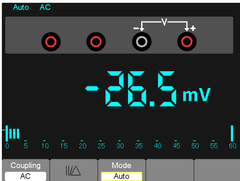
Figure 7-7 AC voltage Measurement
