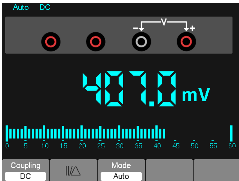
Figure 7-6 DC voltage Measurement
