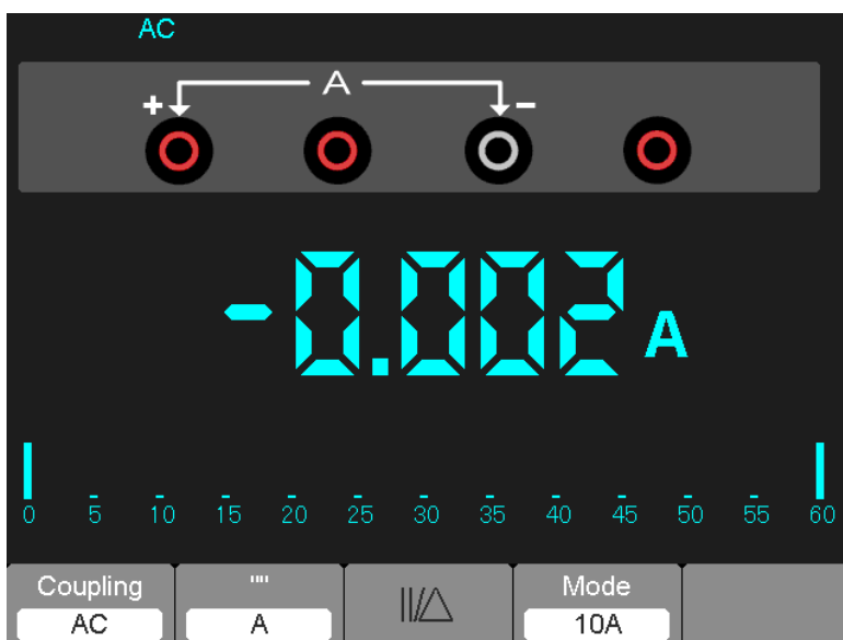
Figure 7-11 AC Current Measurement for 10A
