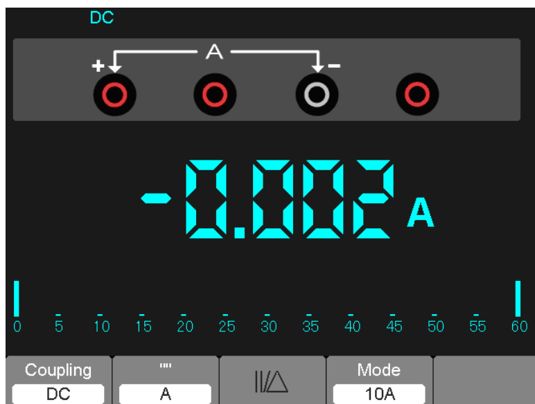
Figure 7-9 DC Current Measurement for 10A
