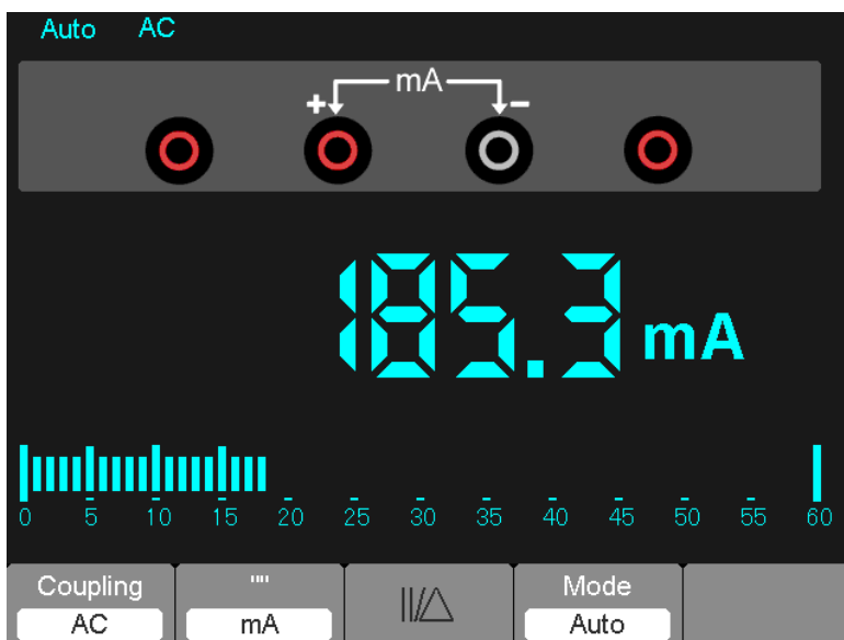
Figure 7-10 AC Current Measurement for 600 mA
