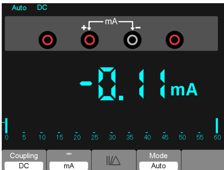
Figure 7-8 DC current Measurement for 600 mA
