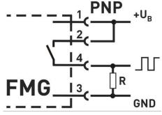
Pull-up- / pull-down-resistors **R**.
