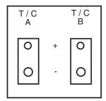
Thermocouple(s) must be fitted with an appropriate compensating standard plug and connected to input T/C A and/or T/C B as required. When using an external cold junction (e.g. ice referencing), copper-copper (not compensating) plugs should be used.
