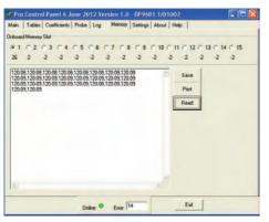
In this tab, readings stored on board the instrument can be retrieved and saved to file (normally in the same folder which contains the PC software).
