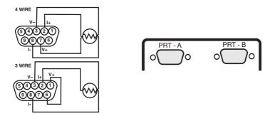
RTDs (Platinum resistance thermometers) must be fitted with a high quality D-plug and connected to input PRT-A and/or PRT-B as required. A 3 or 4 wire configuration can be used but they are connected differently as shown. The instrument will automatically sense which configuration is employed.
