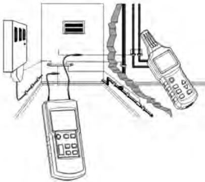
Fig 10. Locating a cold (left) or hot (right) metal water pipe
