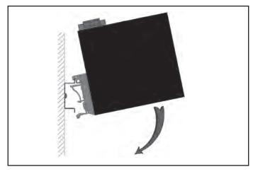
To remove the unit from the DIN rail, place a flat head screwdriver into the release clip found at the bottom of the unit, and apply downward force on the clip until it disengages the bottom of the unit from the DIN rail. Rotate the bottom of the unit towards you and up at an approximate 15° upward angle to completely remove the unit.
