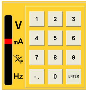
Here the button function of all the functions under OUTPUT (SOURCE) mode are the same as the ones of iCal's numeric buttons.
