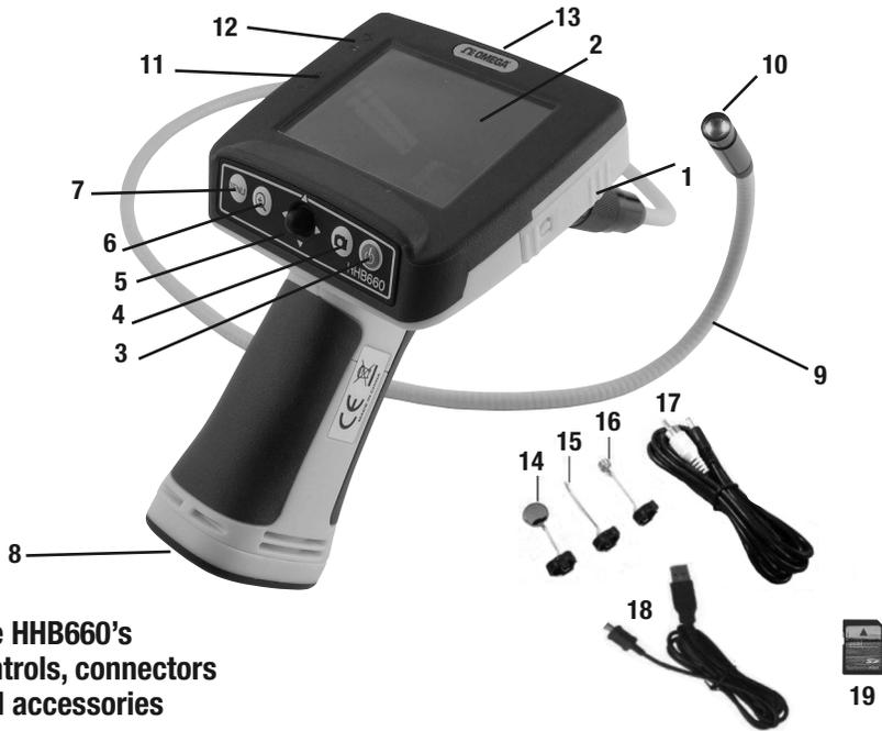
**Fig. 1. The HHB660's controls, connectors and accessories**
