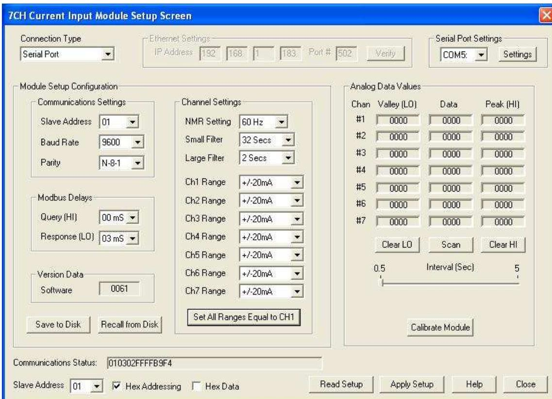
Once the new module configuration settings have been changed to meet the application requirements then press the “Apply” button to transmit the new settings.
