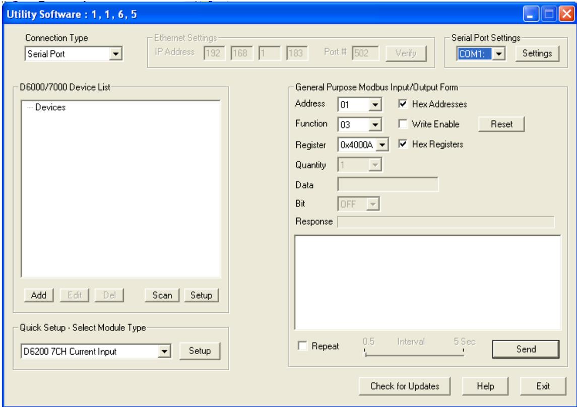
If the "Default\*" line is connected to ground then select 9600 baud, no parity, eight data bits, one stop bit, RTS Only handshaking and the Tx and Rx delays can be left in their default state. Otherwise, adjust the communications settings to match the settings in the connected module.
