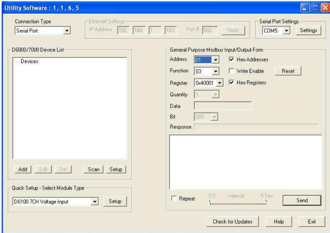
The figure above illustrates the Modbus function 03 being sent to Modbus Slave address 01. Both the command and response messages are displayed beginning with CMD and RSP respectively. This display format is provided for troubleshooting purposes as it displays each byte of information being sent to and received from the module. This format can be a good troubleshooting tool or a way to become familiar with the formatting of the Modbus RTU protocol.
