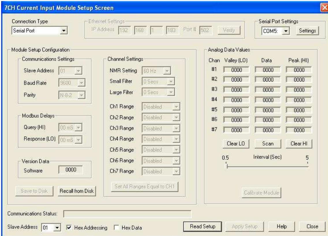
Ensure that the Module Address in the lower left corner is 01 and then press the “Read Setup” button. The screen will now populate with the existing configuration data inside the module.
