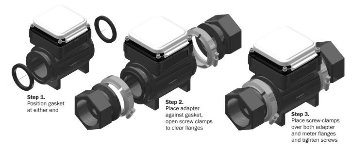
**NOTE:** Above installation instructions are for FMG802/812 (2") and FMG803/813 (3") only. The FMG801/811 (1") is provided with intergrated NPT female threaded ends.
