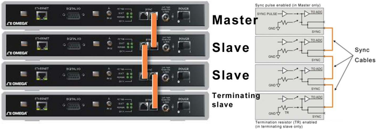
Figure 4. OMB-NET6000 Series devices connected for synchronization
