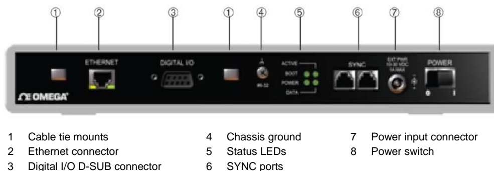
Figure 3. OMB-NET6224 rear panel components
