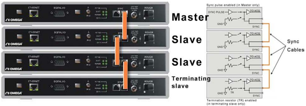
Figure 4. OMB-NET6000 Series devices connected for synchronization
