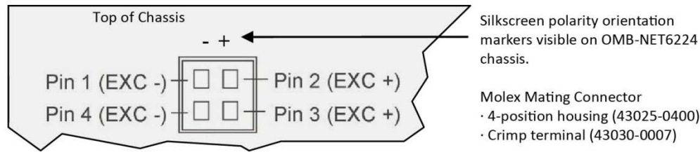
Figure 15. OMB-NET6224 external excitation voltage source pinout
