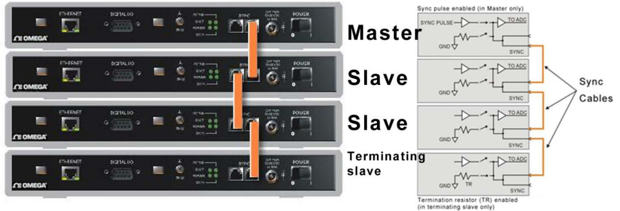
Figure 6. OMB-NET6000 Series devices connected for synchronization
