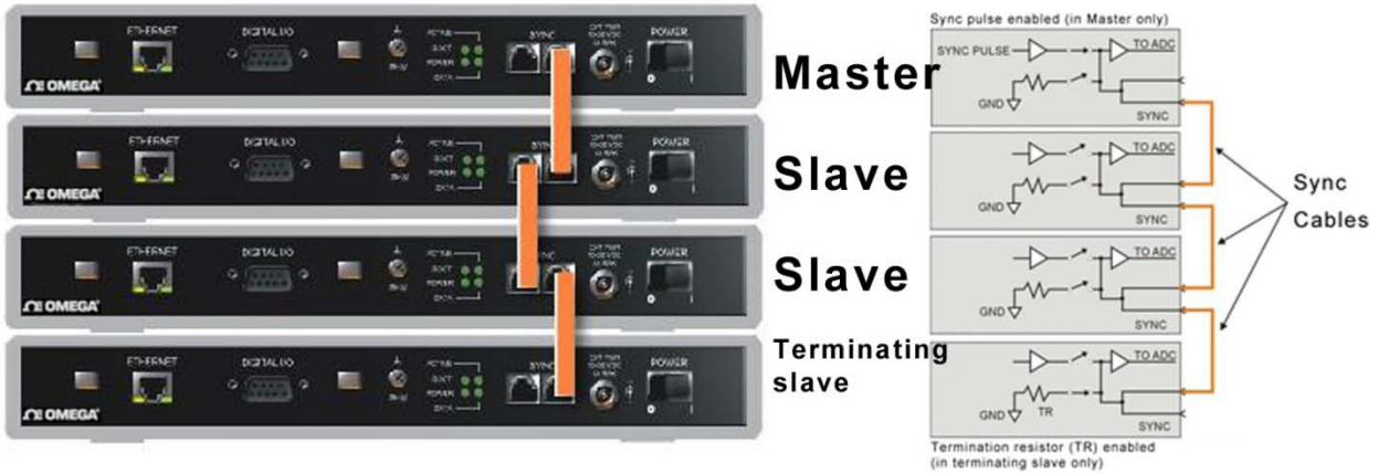
Figure 4. OMB-NET6000 Series devices connected for synchronization
