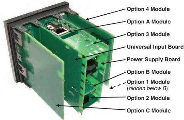
To access the option modules, first pull the instrument from the housing.
