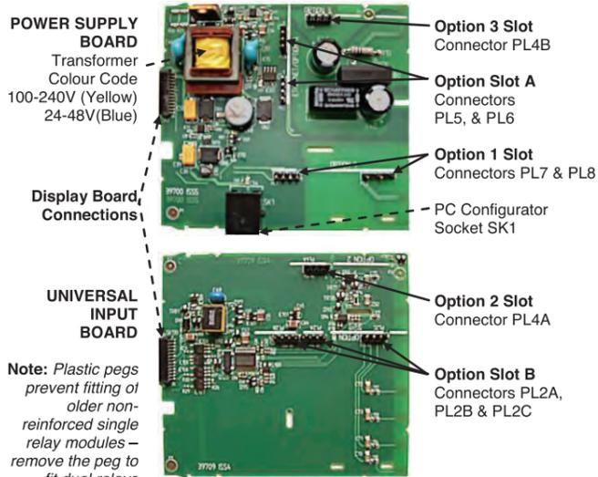
**Note:** Plastic pegs prevent fitting of older non-reinforced single relay modules - remove the peg to fit dual relays
