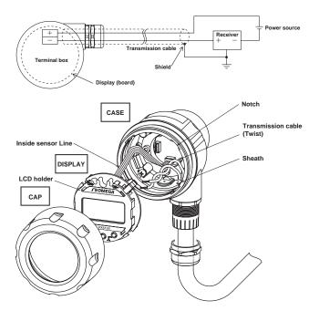
• Turn display over to expose terminal strip, make positive and negative connections, insert wire depth is equal to recommended strip length (0.25").
