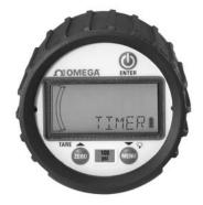
Determines how long the back light will remain ON after any key is pressed in Measurement or Menu Modes (Note: The timer is reset with any key being pressed.)
