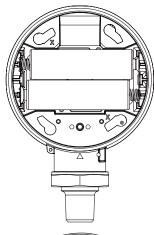
For reattachment of cover, align the 'unlock' icon with the arrow, push cover straight in then turn clockwise until the arrow is in alignment with the 'Lock' icon.
