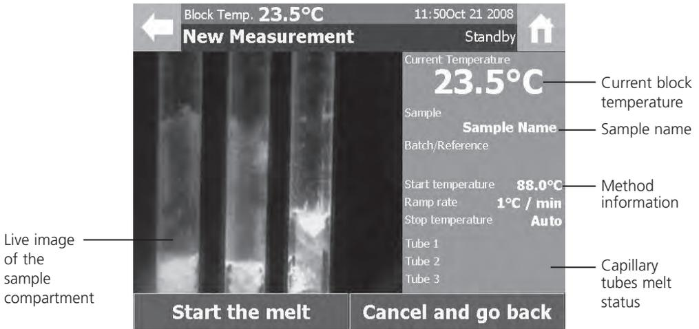
Figure 6: New Measurement Screen
