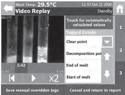
2 Select the timeframe in the video file, where the manual event is to be added, using the video replay scrollbar and the video controls.
