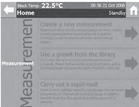
**Create a new measurement:** This option allows a new melt determination to be started. Measurement parameters such as the Sample Name, Start Temperature and Ramp Rate need to be entered when using this option.
