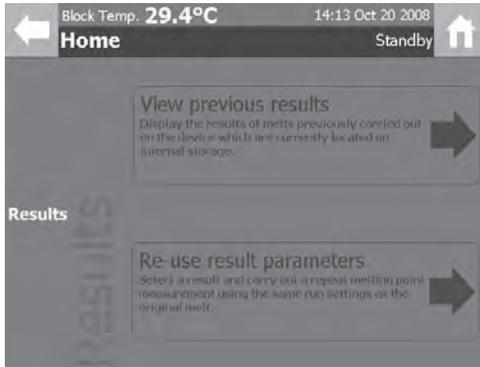
**View previous results:** Displays the result files of melt determinations previously carried out on the device which are currently located on internal storage.
