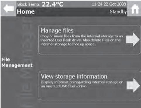
**Manage files:** Result files can be copied, moved or deleted from the devices internal storage.
