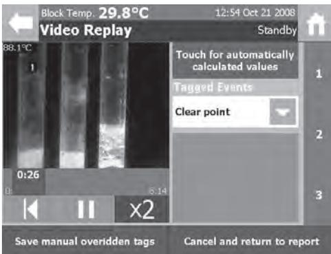
4 Pressing the X2 button will double the speed at which the video is replayed.
