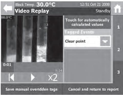
1 Select the capillary tube to which the manual event is to be added by pressing the relevant “Capillary selection” button.
