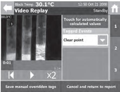
1 To start the video replay press the play button (▶) in the video replay controls. Once the play button has been pressed it will change to a pause symbol (⏸).
