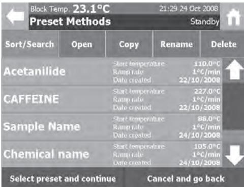
1 In the preset methods screen select the method to be used for the melt determination by pressing on the method details.
