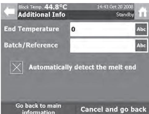
5 Method parameters can be adjusted if required. The SMP40 will automatically detect the end of the melt when the toggle selection field has an X in the “Automatically detect the melt end” field. Removing this check mark allows a value to be entered into the End Temperature field.
