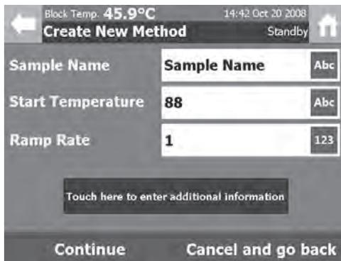
3 Method parameters such as the Sample Name, the Start Temperature and the Ramp Rate can then be adjusted if required by selecting the relevant field.
