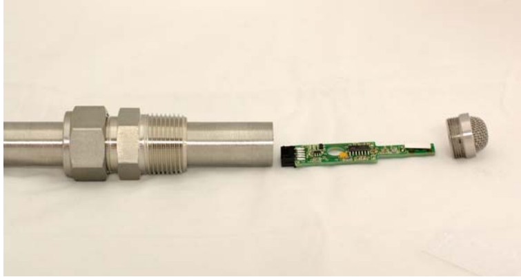
Sensor exploded view for the HX85A or HX86A series
