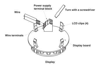
Power Supply Requirements: Although the 4-20mA signal can travel over long distances, a very common issue to arise involves inadequate power at the pressure transmitter – this results in voltage drop across the loop. Be sure to review the accompanying table to determine whether the 12-36Vdc has been received at the pressure transmitter.
