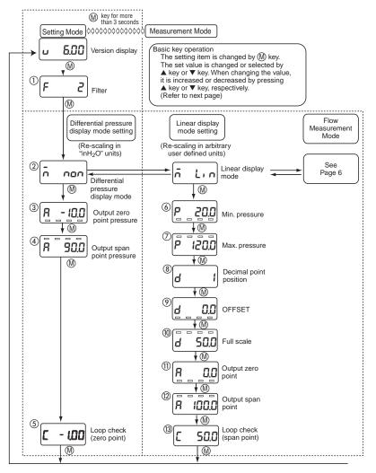
E. Loop Check: Use to send a 4-20mA signal meant to simulate applied pressure, can be accessed either through Pressure Display Mode or Linear Display Mode. See "Complete Setting Mode Menu"; Loop Check is noted on the screen with a prefix "<sup>C</sup><sub>L</sub>". The display is indicating in actual units and starts at the zero (4mA) point.
