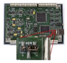
Figure 6. W34 jumper location (default pull-down setting shown)
