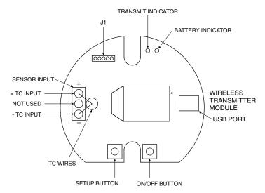
Figure 3-1. Main Transmitter Board
