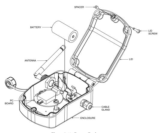
Figure 5-13. Battery Replacement
