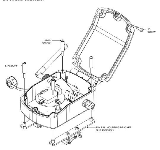
Figure. 5-12. DIN Rail Mounting Bracket Installation
