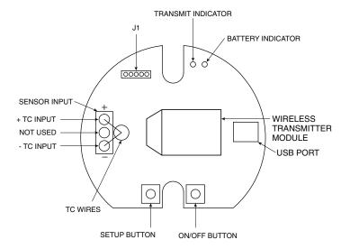
Figure 5-2. Main Transmitter Board
