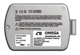
Figure 1-3. UWTC-2A-NEMA, Rear View
