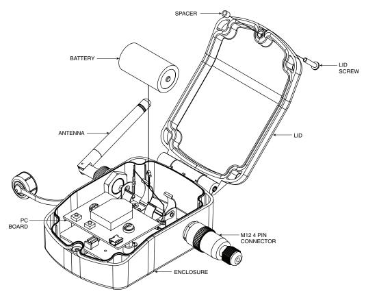
Figure 5-13. Battery Replacement
