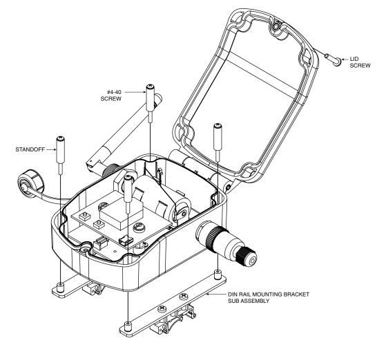
Figure 5-12. DIN Rail Mounting Bracket Installation
