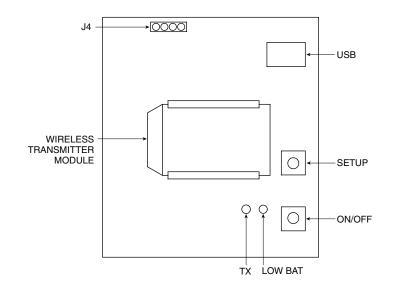
Figure 3-1. Main Transmitter Board
