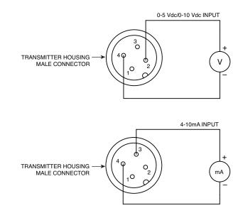
Figure 5-14. Input Diagram for M12 4 Pin Connector
