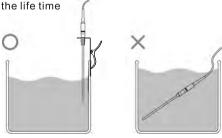
It is suggested you do not hold the probe handle while measuring high temperature. It is better to ues the probe handle for safety.
