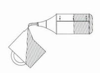
ADD WATER TO BOTTLE WITH BOTTLE IN NORMAL POSITION, FILL TO CALIBRATED MARK
