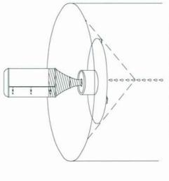
QUICKLY INVERT BOTTLE WITH BASE ATTACHED AND PLACE INTO RAIN GAUGE FUNNEL
