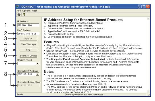
Figure 4.8 Assigning an IP Address using iConnect
