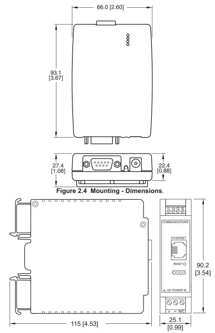
Figure 2.5 DIN Rail iServer Dimensions
