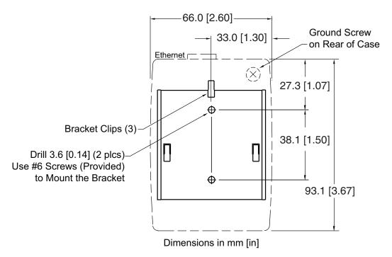
Figure 2.1 Mounting - Wall Mount iServer
