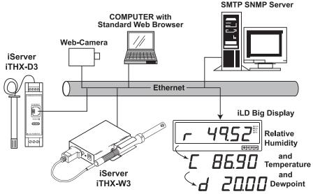
Figure 1.1 iServer with Probe on the Ethernet Network
