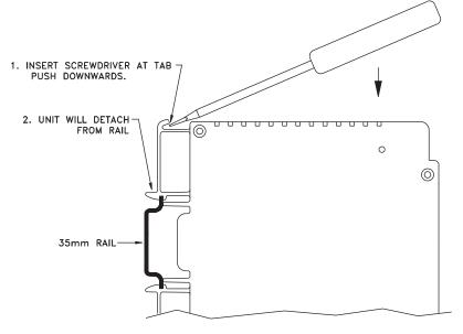
Figure 2.3 Removal - DIN Rail iServer
