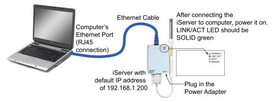
Figure 4.2 Connecting Computer Directly to iServer
