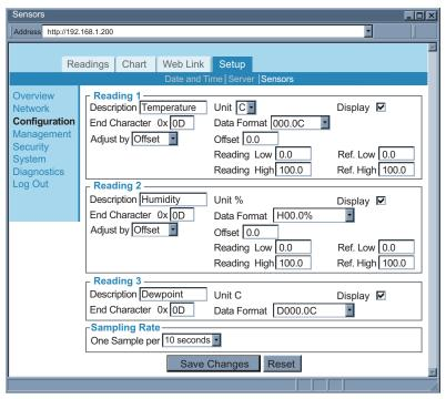
Figure 4.17 Configuration Menu: Sensors
