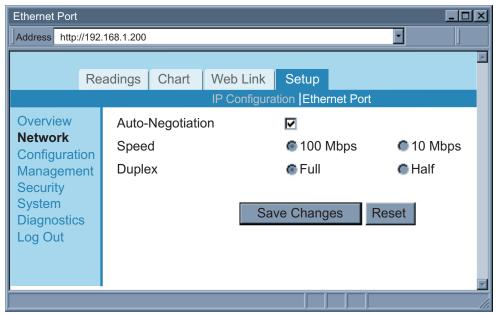
Figure 4.14 Network: Ethernet Configuration
