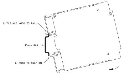
Figure 2.2 Mounting - DIN Rail iServer
