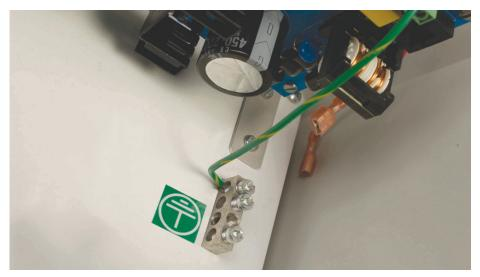
Figure 3-5. Grounding Bus Bar Connection
