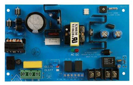
Figure 4-4. HPWS Power Supply
