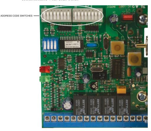
Figure 6-1. Address Codes On HPWS Receiver
