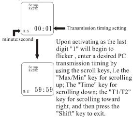
To set the PC transmission timing, the minimum setting time is at one second, and maximum is at 59 minutes and 59 seconds.
