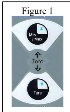
2. To zero the manometer using **Factory Zero**, start with the unit turn **ON** and in **Measure Mode** and use the following keystroke sequence:
