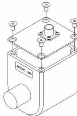
Do NOT immerse the assembly in the solvent. This may damage the strain gages inside the slip ring. Also, do NOT clean the brushes with the solvent.
