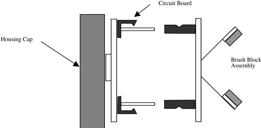
The brush block assembly is keyed to only fit on the circuit board one way.
