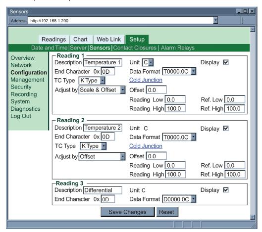
Figure 4.17 Configuration Menu: Sensors
