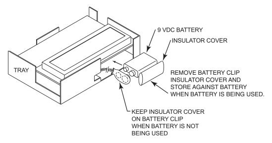
Figure 2.5 Battery Installation
