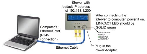
Figure 4.2 Connecting Computer Directly to iServer
