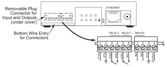
Figure 2.7 Relay and I/O Contact Connections
