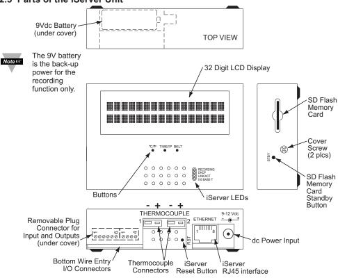
Figure 2.3 Parts of the iServer Unit
