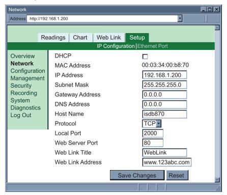
Figure 4.13 Network: IP Configuration
