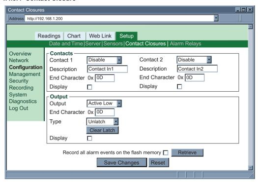
Figure 4.18 Configuration Menu: Contact Closures
