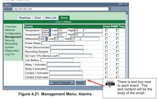
This includes events or conditions. Once a condition is met the iServer will send an email or/and an SNMP trap if either one or both are checked. Fields are described below.
