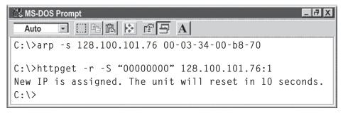
Figure 4.1 ARP and HTTPget Commands on a DOS Window
