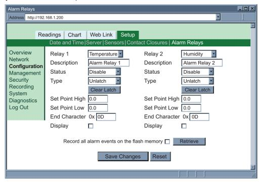
Figure 4.19 Configuration Menu: Alarm Relays
