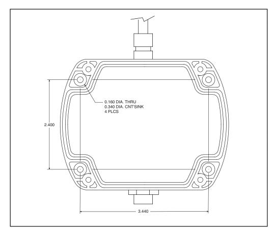
Figure 4. FMA1000 Transmitter Wall Mounting Holes
