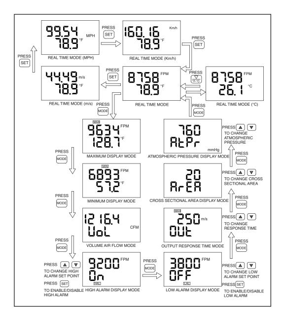
Figure 5. Functional Display Flow Chart
