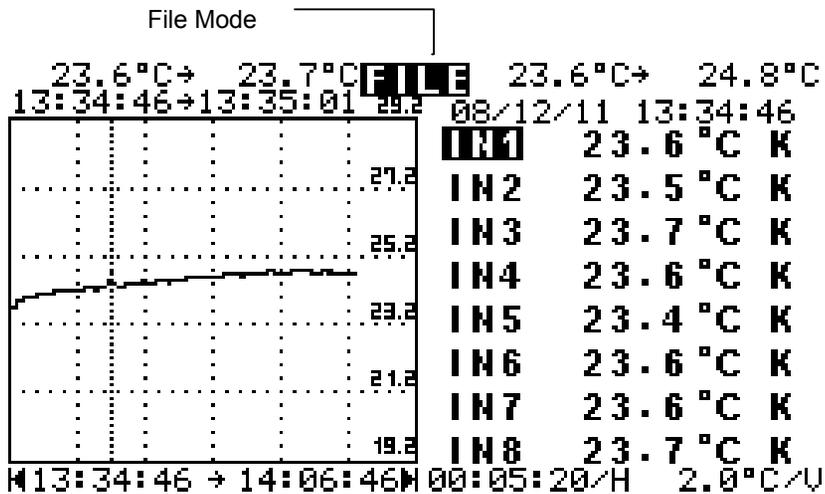
4. Curve of overall trend of all data is shown in the left hand side of LCD.
