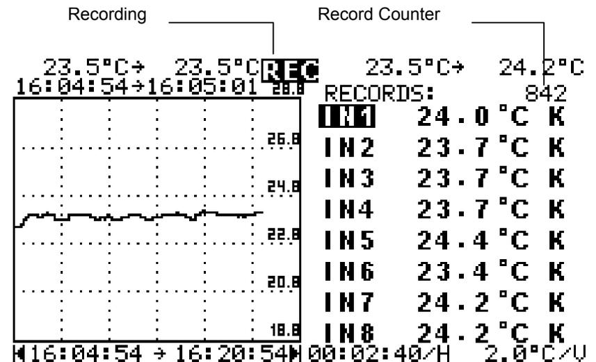
1. Press the REC button to record data. A symbol of "REC" is shown at the top center of LCD.
