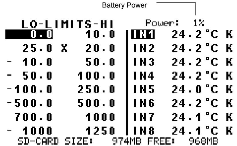
1. When power is turned on, the % (percentage) of battery power is displayed at the right top corner of LCD. If the % is less than or equal to 1%, please replace the batteries with new ones.
