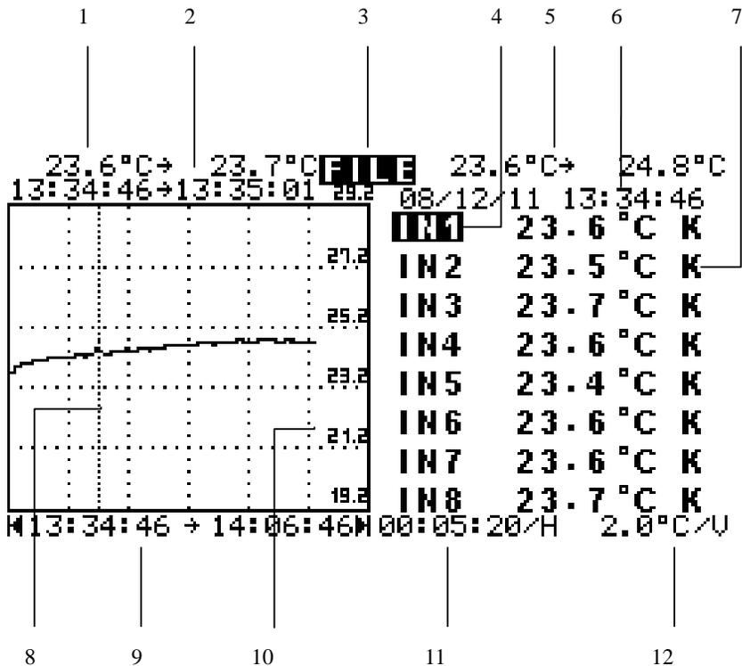
1. Minimum and Maximum Temperature Values during the time interval at the Current Cursor Position
