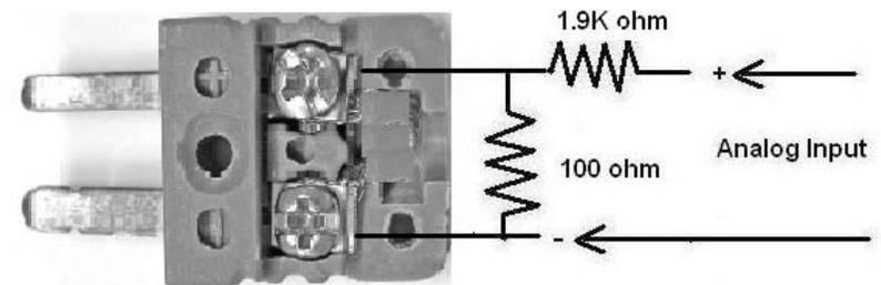
1. The full scale output is 1000 mV per 100 %RH.
