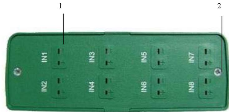
1. **Input for Thermocouple Mini Connector**
